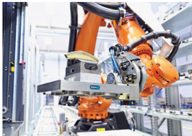
For small and medium-sized lots, the SCHUNK VERO-S NSA plus palletizing system ensures high process reliability and flexibility
